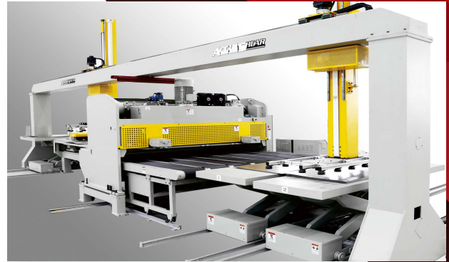
Conveyor, Unloading and Stacker system
